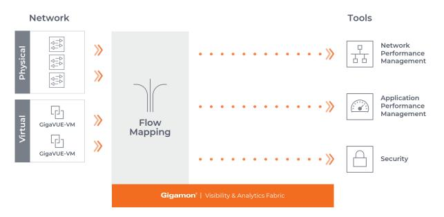
Flow Mapping takes line-rate traffic at 1Gb, 10Gb, 25Gb, 40Gb or 100Gb from a network TAP or a SPAN/mirror port and sends it through a set of user-defined map rules to the tools and applications that secure, monitor, and analyze IT infrastructure
