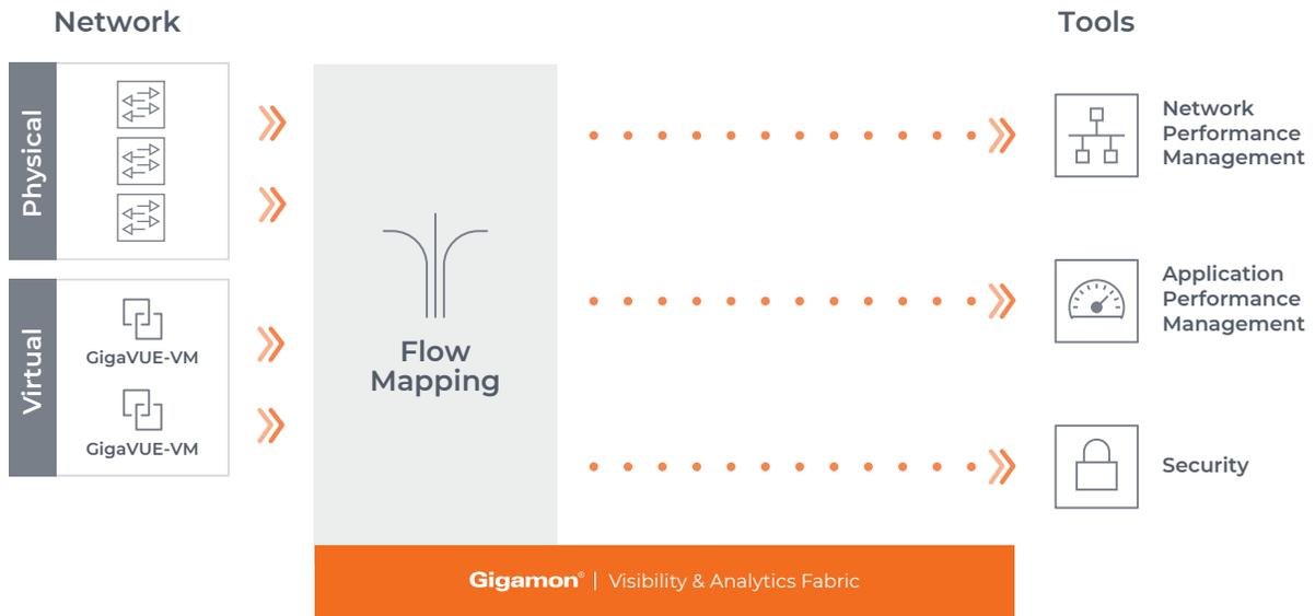
Flow Mapping takes line-rate traffic at 1Gb, 10Gb, 25Gb, 40Gb or 100Gb from a network TAP or a SPAN/mirror port and sends it through a set of user-defined map rules to the tools and applications that secure, monitor, and analyze IT infrastructure
